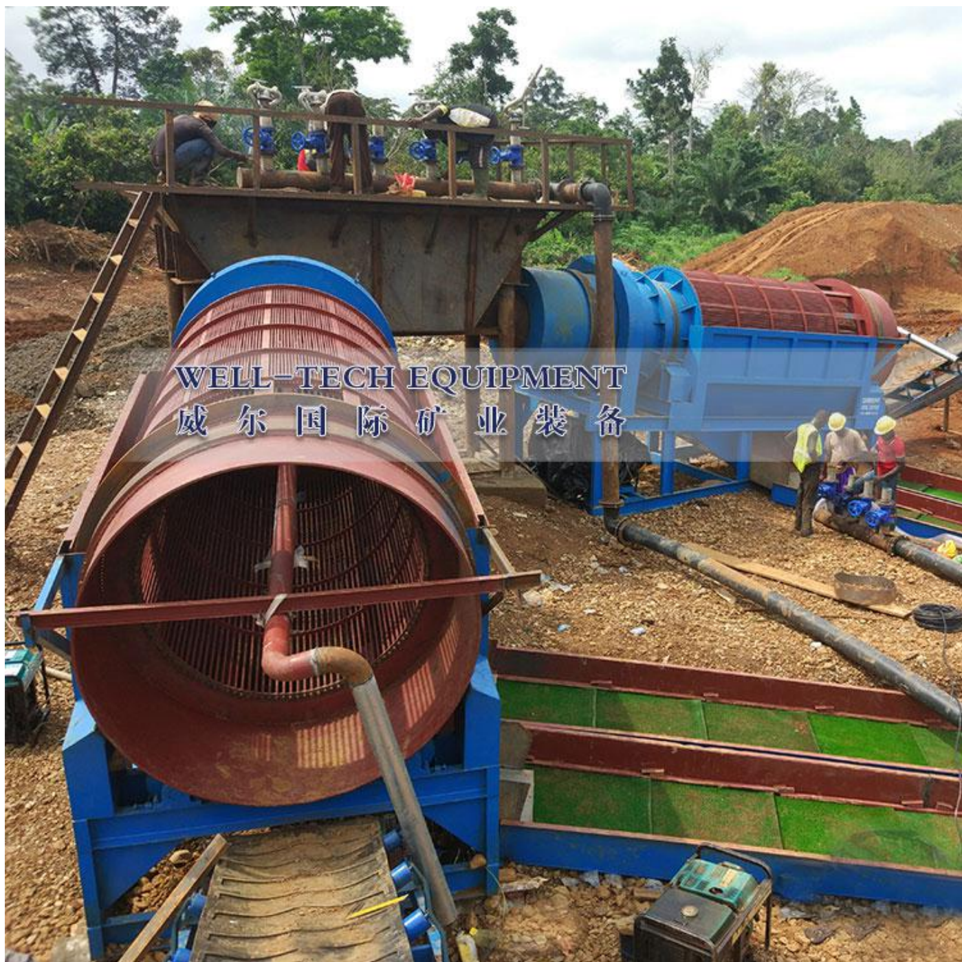
Gold trommel wash plant in Africa
